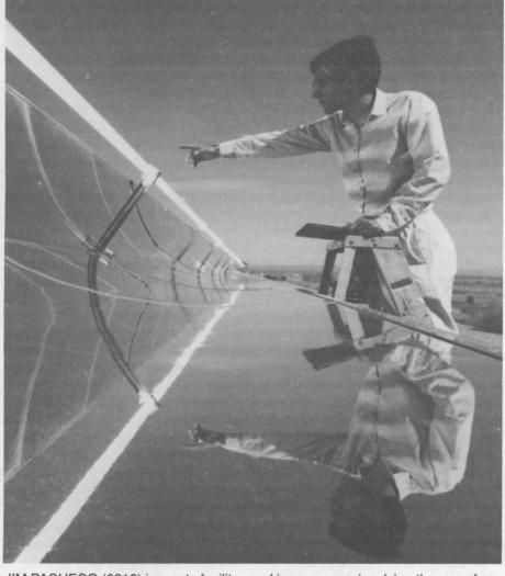
JIM PACHECO (6216) inspects facility used in a program involving the use of solar energy to destroy toxic wastes in water and organic wastes.
